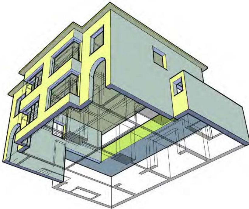
Fig 2 A plan is a 2-D representation of a building as seen from above. The ground floor plan is like the 'footprint' of the building; it is the key to understanding its function.
