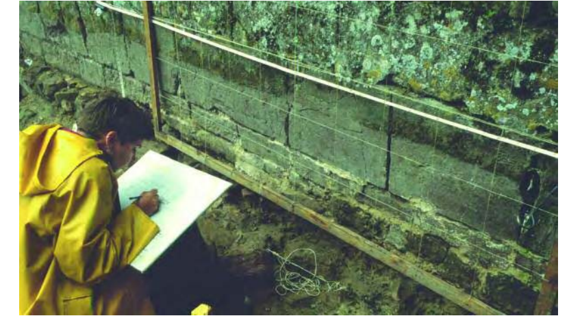
Fig 26 Recording a wall using a rigid recording frame.
