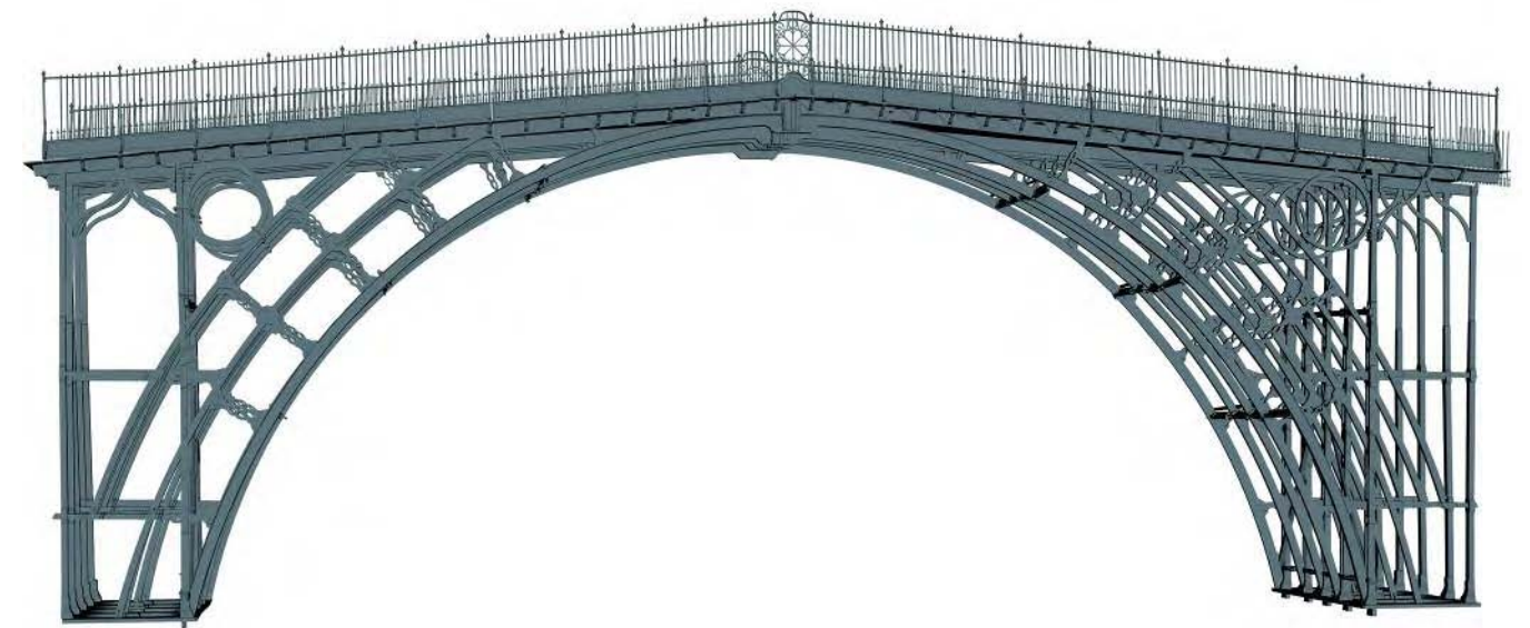
Fig 61 View of the CAD model matched to the view of the Iron Bridge shown in Fig 60 and revealing the casting error on frame C.
