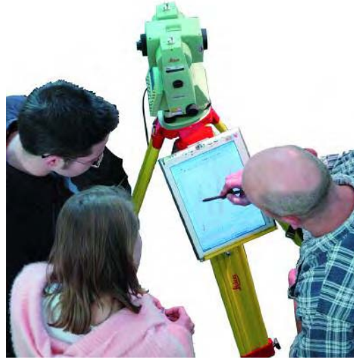
Fig 24 Real-time CAD set-up in use: the tablet PC makes it possible to see and check the CAD work as the data are captured, a useful method for detail work using a TST.
