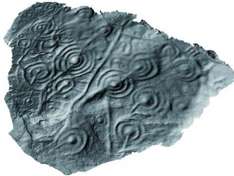
Fig 21 Triangulation scanner data: small, smooth-surfaced objects make good subjects for triangulation scanners. Laser scanning can support the study of rock art by providing rapid, standardised data sets of scattered objects, aiding the distributed analysis of carved patterns of this kind. Sculptural details can be captured successfully using such scanners, but getting the scanner to the subject on a stable platform can be a challenge.
